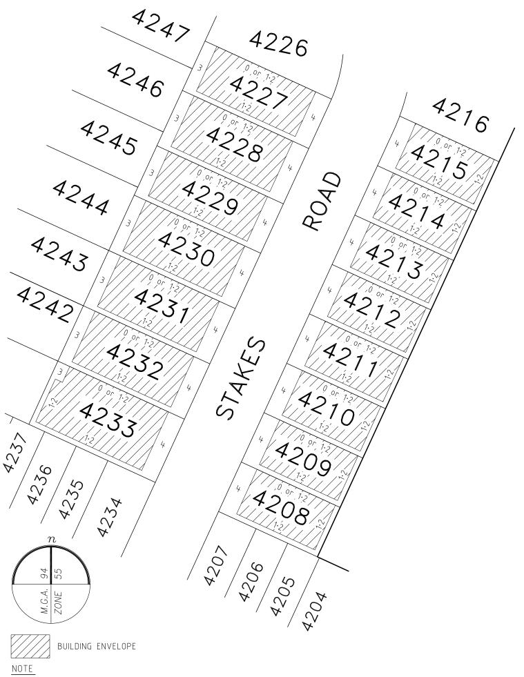
THE BUILDING ENVELOPE OF LOT 4233 IS PARTIALLY DEFINED BY EASEMENT BOUNDARIES. FOR FULL LOT & EASEMENT DIMENSIONS REFER TO SHEET 3 ON PS845596Y.
